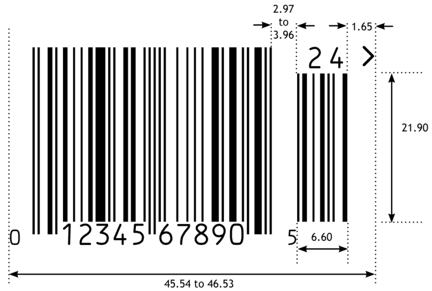
Figure 5.2.6.6-5. UPC-A barcode with two-digit add-on symbol
